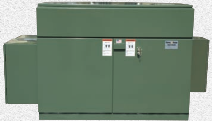
Figure 1. Exterior view of FP Automatic-Transfer, Pad-Mounted Switchgear ATPSE-9 shows the motor operator and control compartment on each side. The control compartment contains the FP Automatic Transfer Micro-processor. The FP Switch Operators are in separate compartments. The automatic transfer system provides the customer with two independent power sources to assure service continuity for critical loads. The FP Live-Front Automatic-Transfer Pad-Mounted Switchgear Type ATPSI/II-9 is configured in a similar manner. For views of switch and fuse compartments for FP Live-Front Pad-Mounted Switchgear refer to pages 9 and 11 for FP Dead-Front Pad-Mounted Switchgear refer to pages 31-33.
